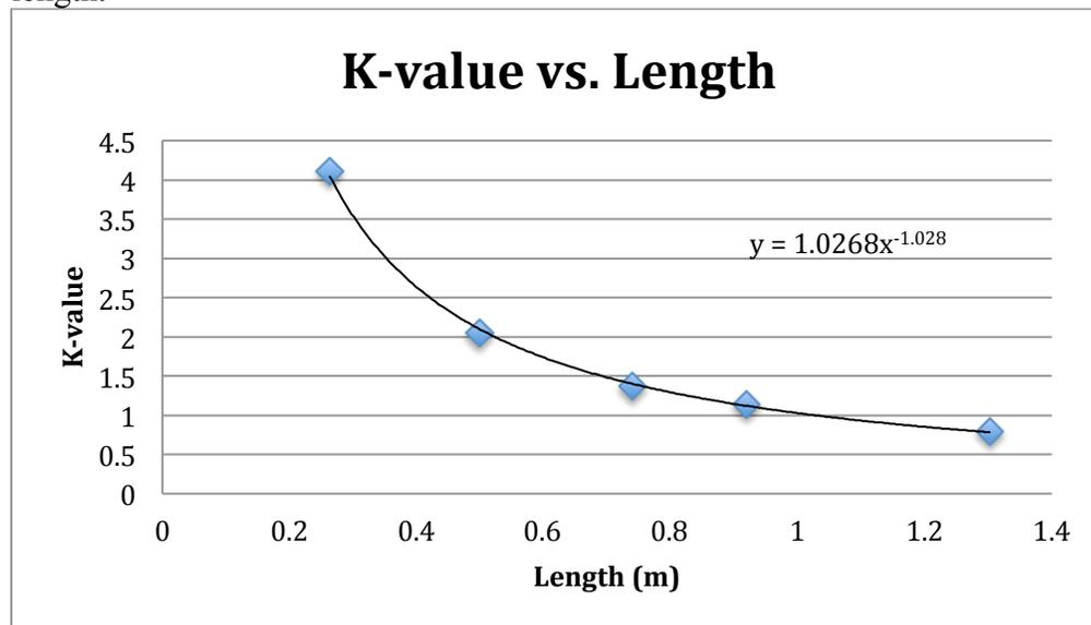
Figure 8: K-value vs. 1/Length. The equation for this graph gives the linear relationship our bungee cord's elastic constant and 1/Length.
