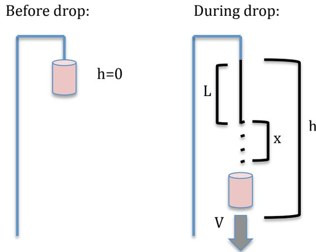
**Figure 1. Set-up for dropping mass and measuring vertical displacement.** In this set up, we used a constant hanging mass ( $m$ ), varied the cord length ( $L$ ) for each trial, and measured the maximum length of the fall, which we deemed as the height ( $h$ ) of the system. We could then determine displacement ( $x$ ) by subtracting length of cord from  $h$  ( $x=h-L$ ).
