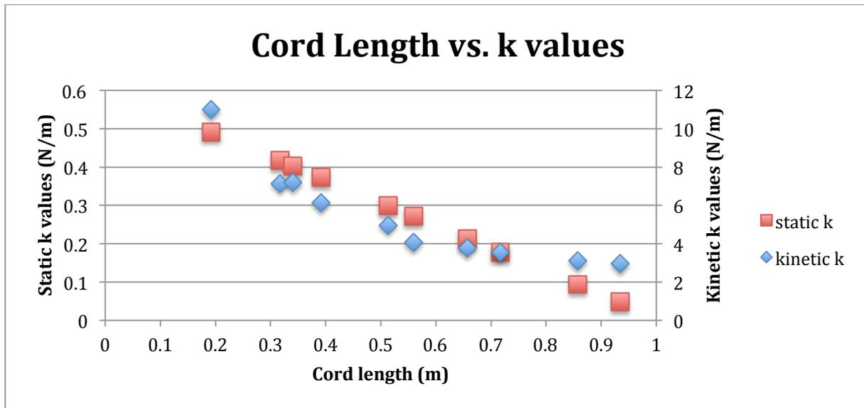
**Figure 2. Comparison of static and kinetic k values based on varying cord length.** Static k values were determined using equation 1 from our static results in *Bungee I*. Kinetic k values were calculated in Table 2.
