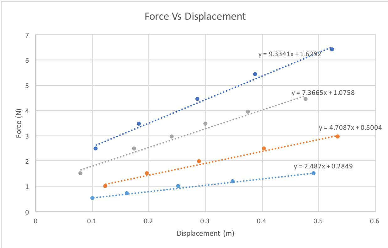
The above graph shows that the relationship between force applied and displacement from equilibrium is linear, as expected by Hooke's law  $F=kx$ . The lowest line, the light blue one, represents 1 cord, the orange line represents 2 cords, the grey represents 3 cords, and the dark blue represents 4 cords.
