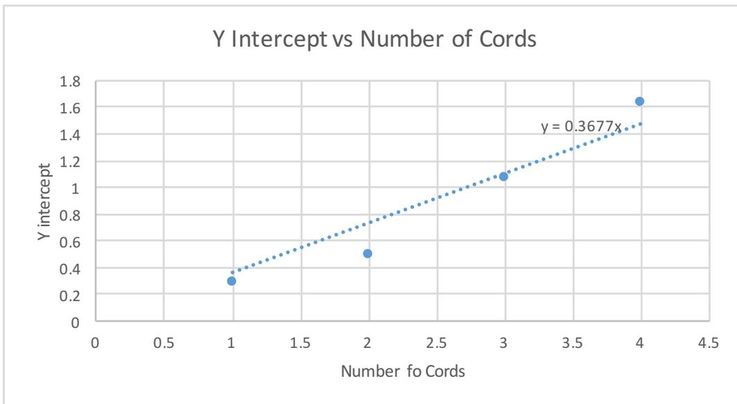
The above graph attempts to determine a relationship between the y intercepts of each curve and the number of cords. It can be seen that the relationship is not quite linear, however there is an upward sloping trend. The experimental value of interest is also the coefficient of the x term.
