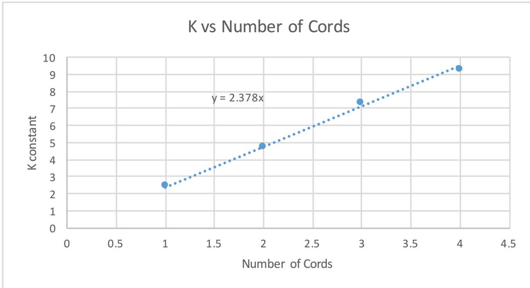
The above graph shows the relationship between K constant and the number of cords in the system. It can be seen above that the relationship is quite linear. The value of interest in the above graph is the coefficient on the x term.
