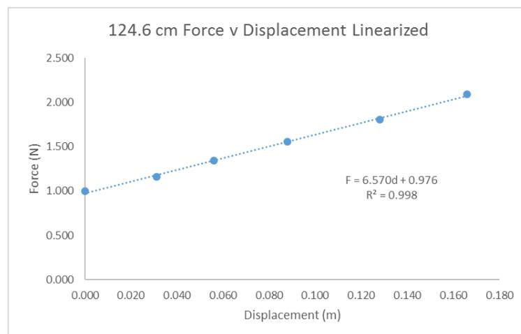
Figure 9: The linearized force as a function of displacement when mass is applied to a double strand with a length of 124.6 cm (1.246 m). The conditions result in a spring constant of 6.570 and the relationship is functionally linear with an  $R^2$  value of .998.
