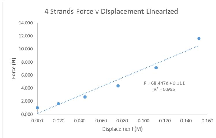
Figure 6: Figure 5: The linearized force as a function of displacement when mass is applied to a quad strand. The conditions result in a spring constant of 68.447 and the relationship does not show a confident level of linearity.
