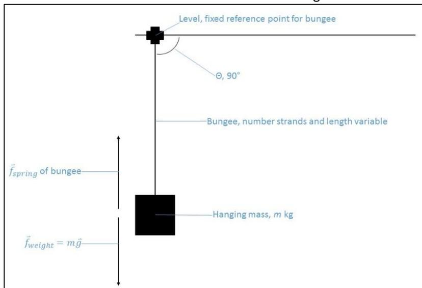
Figure 1: Schematic of the bungee and hanging mass system, include all forces present.
