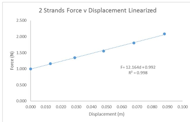
Figure 5: The linearized force as a function of displacement when mass is applied to a double strand. The conditions result in a spring constant of 12.164 and the relationship is functionally linear with an  $R^2$  value of .998.
