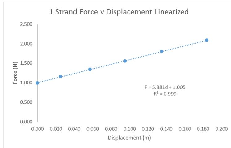
Figure 4: The linearized force as a function of displacement when mass is applied to a single strand. The conditions result in a spring constant of 5.881 and the relationship is functionally linear with an  $R^2$  value of .999.
