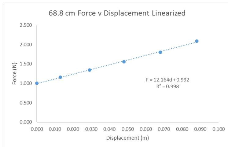
Figure 8: The linearized force as a function of displacement when mass is applied to a double strand with a length of 68.8 cm (.688 m). The conditions result in a spring constant of 12.164 and the relationship is functionally linear with an  $R^2$  value of .998.
