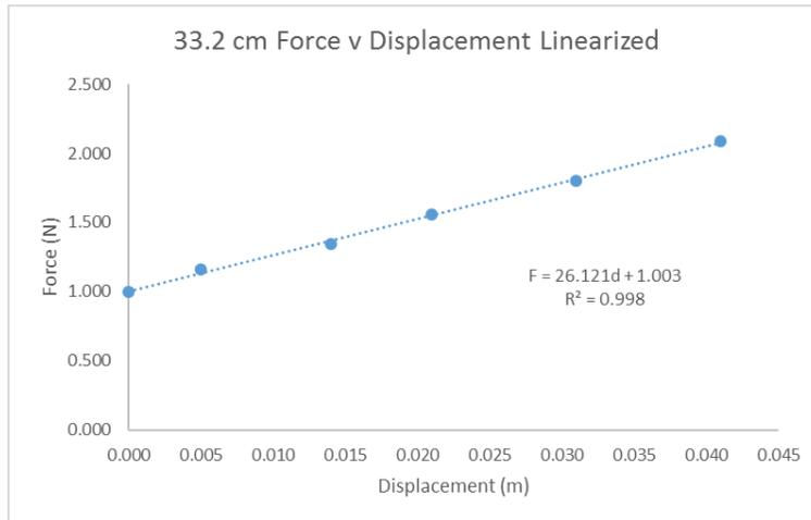
Figure 7: The linearized force as a function of displacement when mass is applied to a double strand with a length of 33.2 cm (.332 m). The conditions result in a spring constant of 26.121 and the relationship is functionally linear with an  $R^2$  value of .998.
