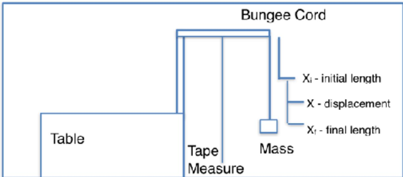
**Figure 1: Bungee and Hanging Mass System.** A bungee is connected to a hanging apparatus and connected to a mass.
