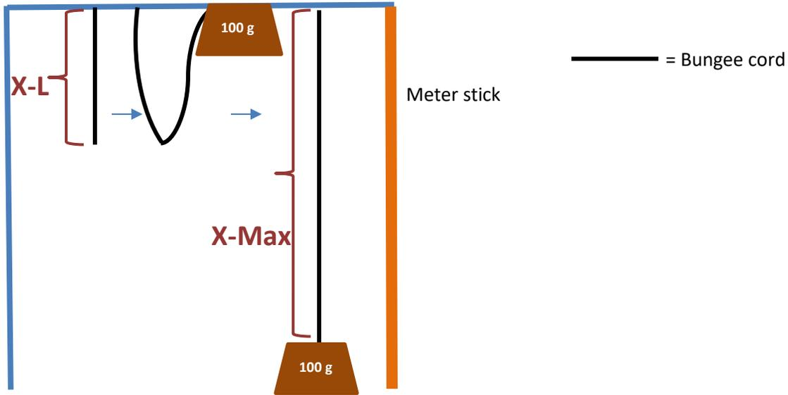
Figure 1. Diagram of experimental set-up with relevant variables.
