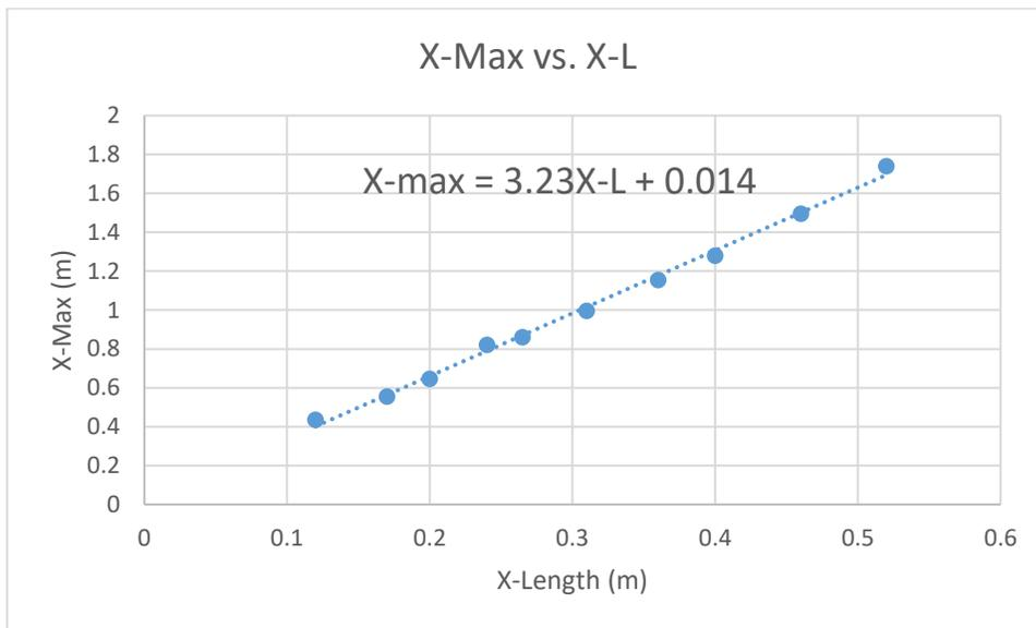
Figure 2. Graph of X-max (maximum bungee stretch after a mass was dropped) versus X-L (initial un-stretched bungee length).
