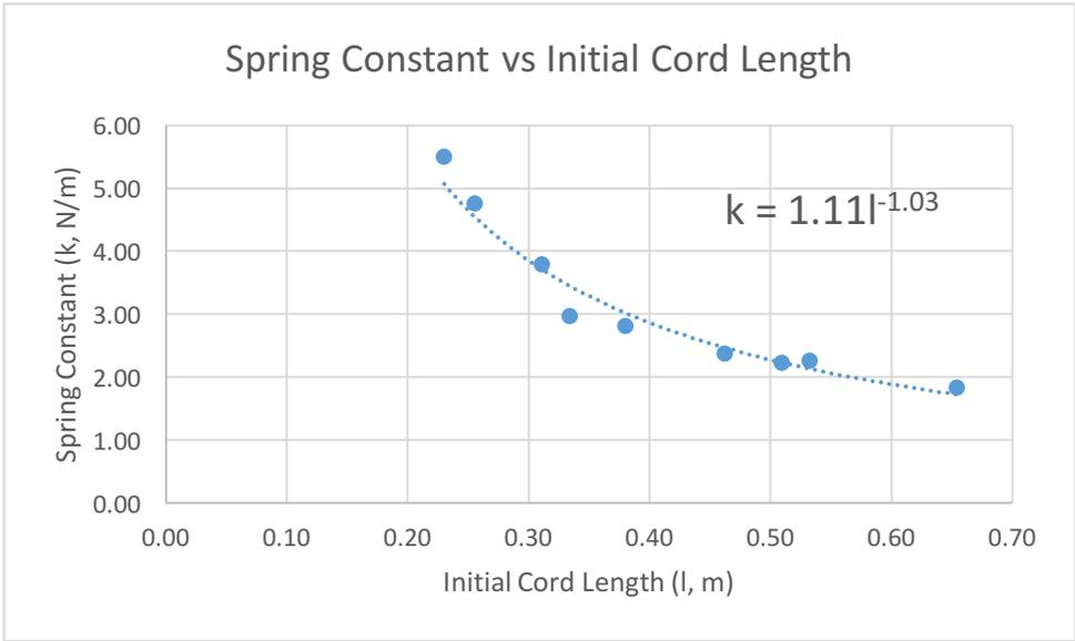
Figure 11: We plot the spring constants against the initial cord lengths. The power-fit equation is  $k = 1.11l^{-1.03}$ .
