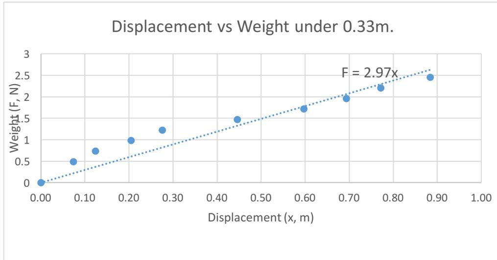
Figure 7: Linearization of displacement and weight based on Hook's Law. The equation is  $F = 2.97x$ . The uncertainty is 5.3% from regression analysis.
