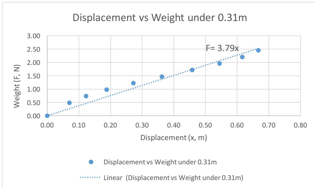
Figure 8: Linearization of displacement and weight based on Hook's Law. The equation is  $F = 3.79x$ . The uncertainty is 3.7% from regression analysis.
