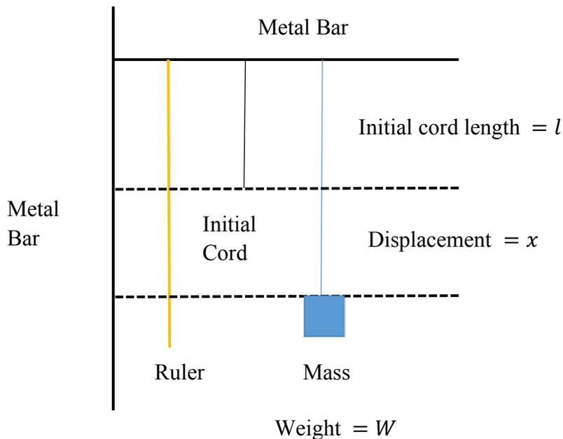
Figure 1: Sketch of setup. The cord and the ruler are attached to the metal bar and fall parallel to each other, perpendicular to the level ground. The mass is added to the hanger at the end of the cord. The hanger is not shown here.
