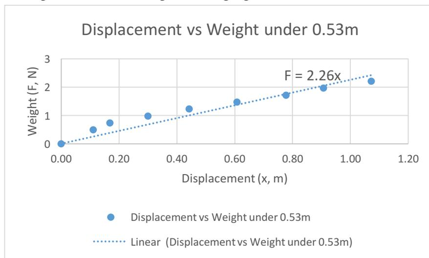
Figure 3: Linearization of displacement and weight based on Hook's Law. The equation is  $F = 2.26x$ . The uncertainty is 5.4% from regression analysis.
