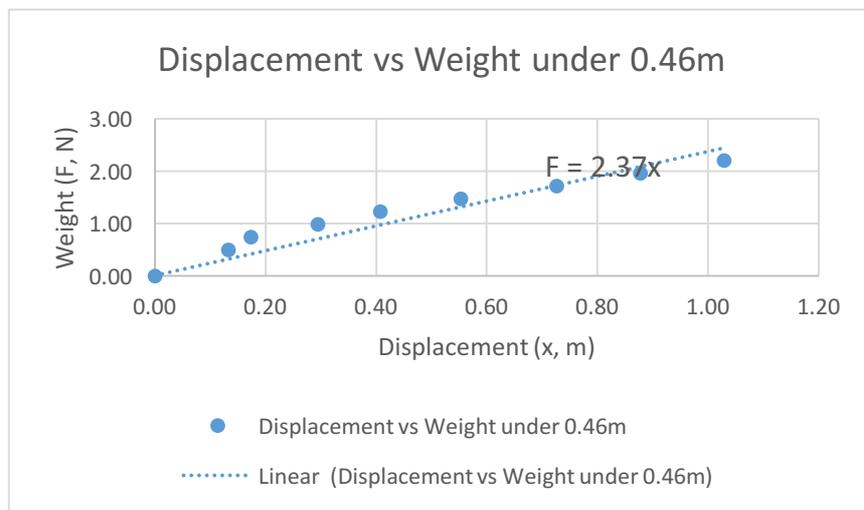
Figure 5: Linearization of displacement and weight based on Hook's Law. The equation is  $F = 2.37x$ . The uncertainty is 5.3% from regression analysis.
