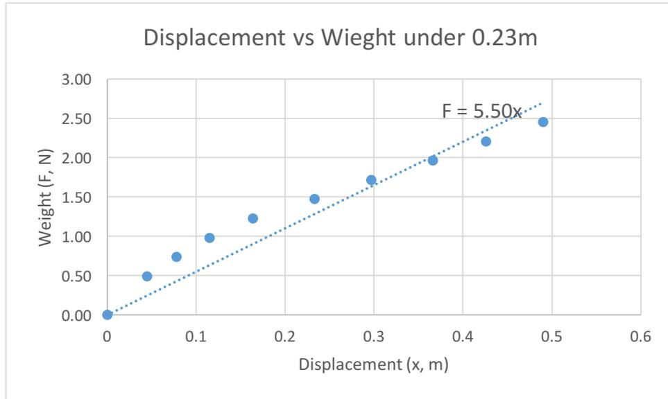
Figure 10: Linearization of displacement and weight based on Hook’s Law. The equation is  $F = 5.50x$ . The uncertainty is 4.9% from regression analysis.
