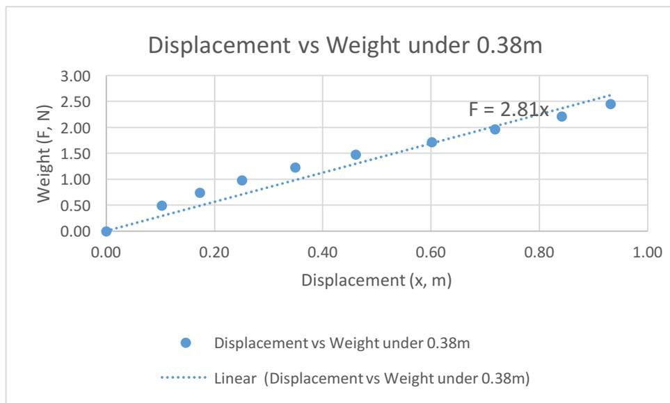
Figure 6: Linearization of displacement and weight based on Hook's Law. The equation is  $F = 2.81x$ . The uncertainty is 4.0% from regression analysis.
