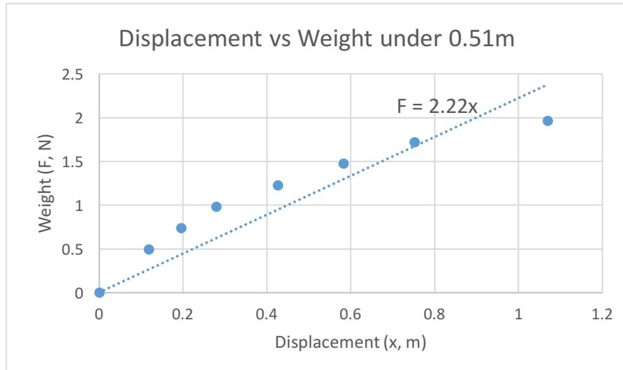
Figure 3: Linearization of displacement and weight based on Hook's Law. The equation is  $F = 2.22x$ . The uncertainty is 8.2% from regression analysis.
