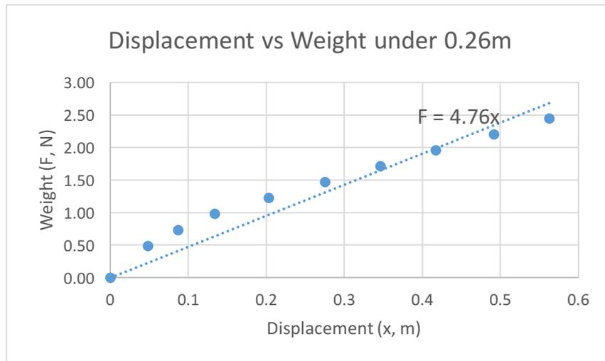
Figure 8: Linearization of displacement and weight based on Hook’s Law. The equation is  $F = 4.76x$ . The uncertainty is 4.7 from regression analysis.
