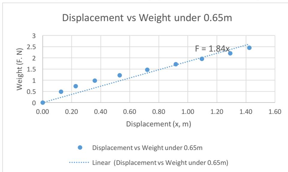
Figure 2: Linearization of displacement and weight based on Hook's Law. The equation is  $F = 1.84x$ . The uncertainty is 4.4% from regression analysis.
