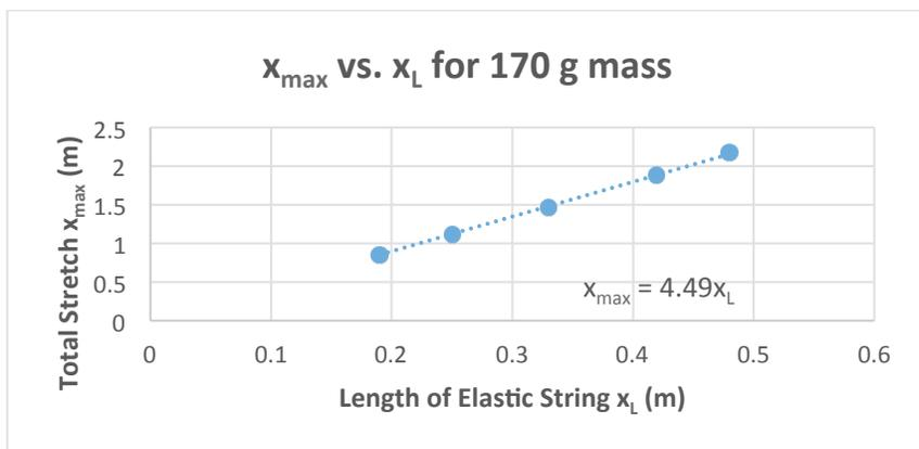
**Figure 5: Graph of  $X_{\max}$  vs.  $X_L$  for the 170 g mass. The “fall factor” is 4.49**
