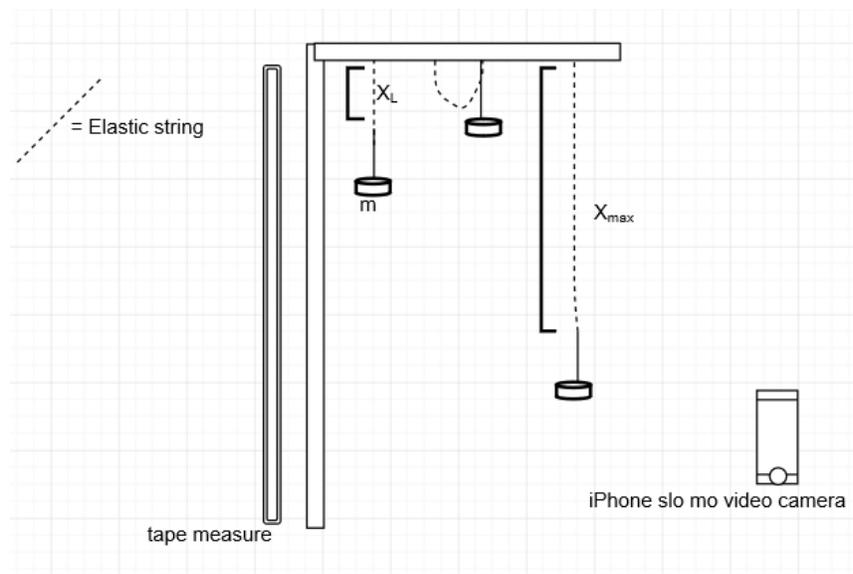
**Figure 1: Methods Diagram.** Basic setup with variables and important details.
