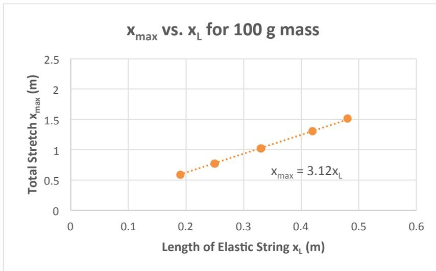
**Figure 3: Graph of  $X_{\max}$  vs.  $X_L$  for the 100 g mass. The “fall factor” is 3.12.**
