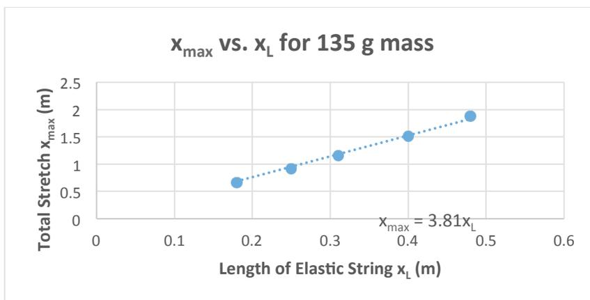
**Figure 4: Graph of  $X_{\max}$  vs.  $X_L$  for the 135 g mass. The “fall factor” is 3.81.**
