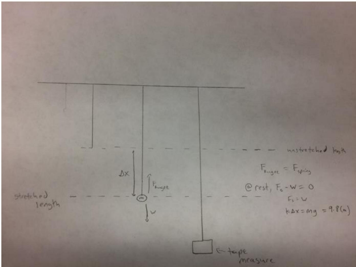
**Figure #1, Diagram of our experimental setup**
