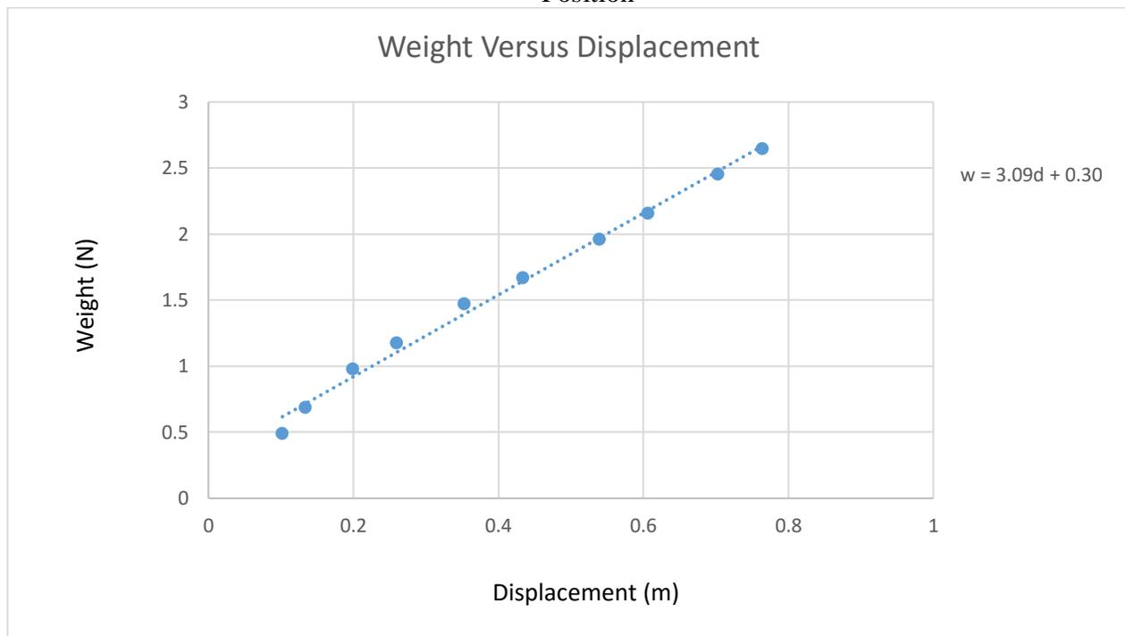
This graph displays the weight of the hanging masses versus the displacement of the bungee cord sample. The slope of the graph is an approximation of  $k$  for the cord.
