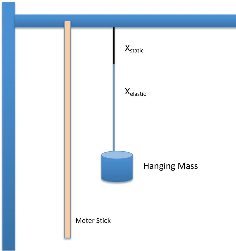
**Figure 1: Diagram of Setup.** This diagram shows how the static and elastic cords were attached to form the total cord.
