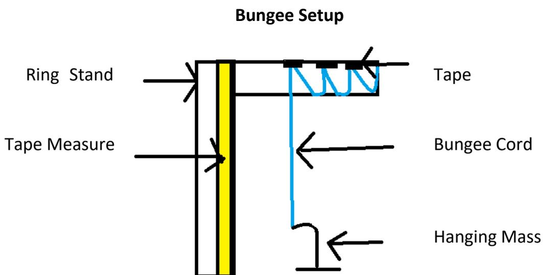
**The diagram above demonstrates the setup for the bungee lab when the bungee cord is at its maximum distance.**
