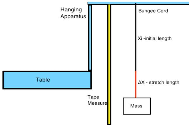
**Figure 1:** Diagram of the experimental design. Masses were dropped from the top of the hanging apparatus and displacement was measured using a slow-motion camera at the lowest point of the fall. Hanging mass in the diagram is at lowest point in fall where the  $P_e$  of the bungee is greatest.
