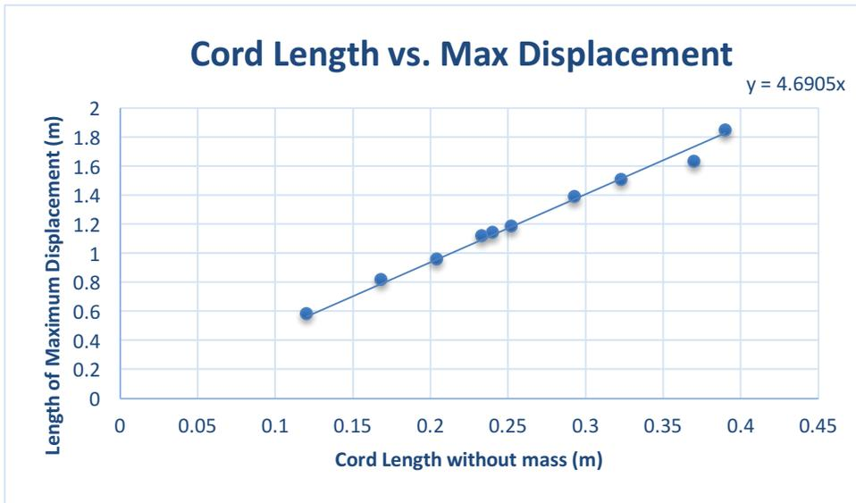
The linearized equation is  $X_{max} = 4.7X_L$ , where  $X_{max}$  represents the cord's maximum displacement during the fall,  $X_L$  represents the length of the cord without the hanging mass, and 4.7 represents the spring constant,  $k$ .
