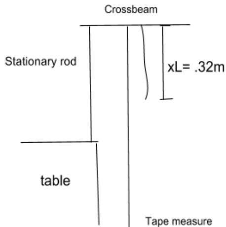
**Figure 1:** The diagram shows the crossbeam with the tape measure stretched from the crossbeam to the floor and the unstretched bungee.
