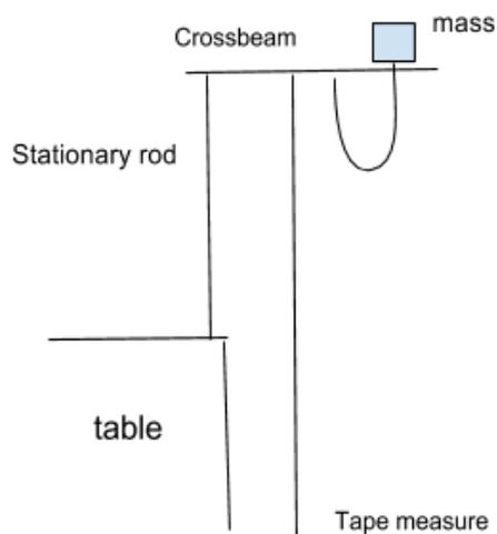
**Figure 2:** This diagram shows the set-up of the experiment right before we drop the mass. We hung the mass so that the bottom of the mass was right above the crossbeam.
