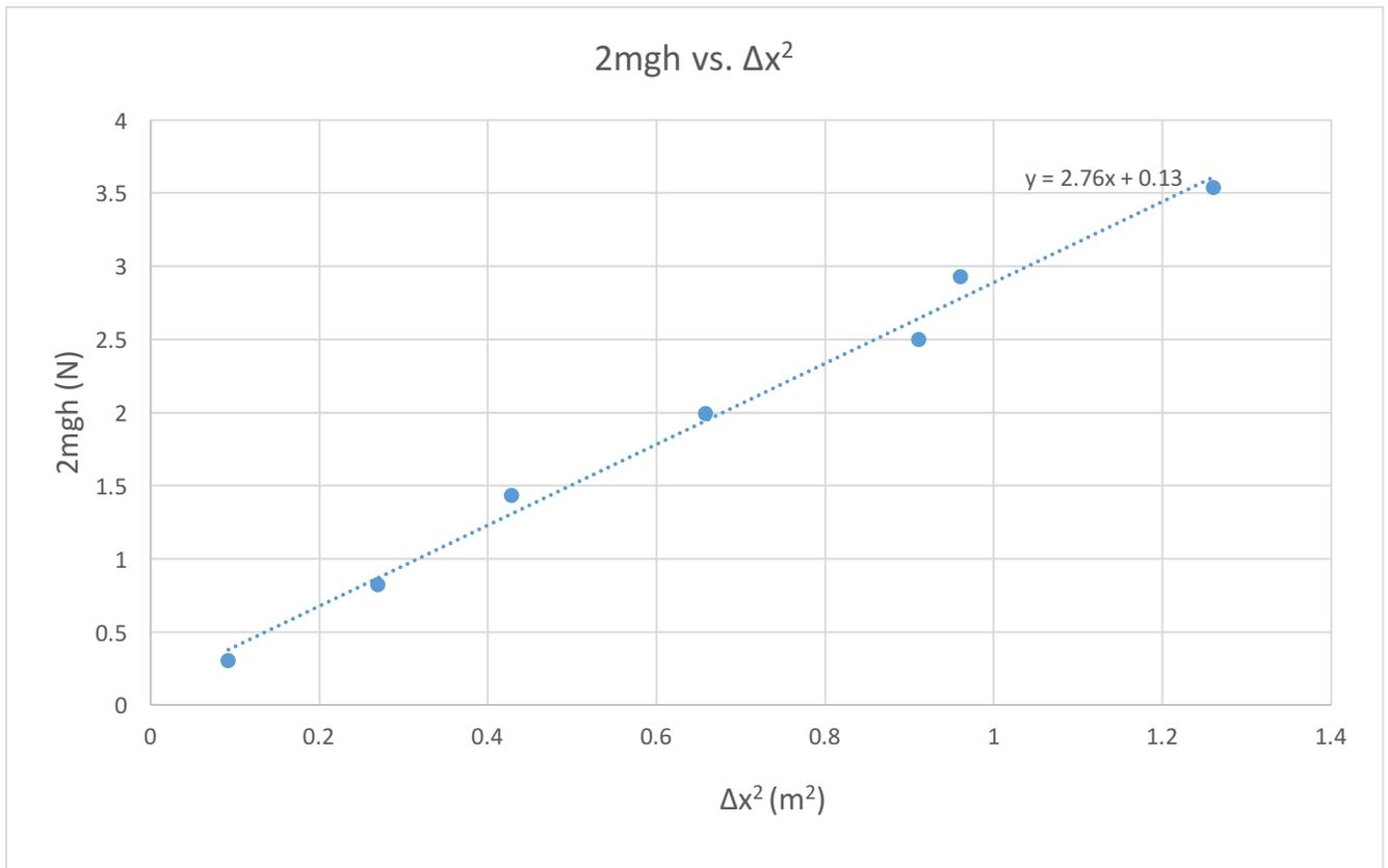
**Graph 1:** The Potential Energy, Doubled, vs. the Change in X, Squared, of the Mass. The slope,  $2.76 \pm 0.12 \text{ N/m}^2$  is the value  $k$  of the bungee cord.
