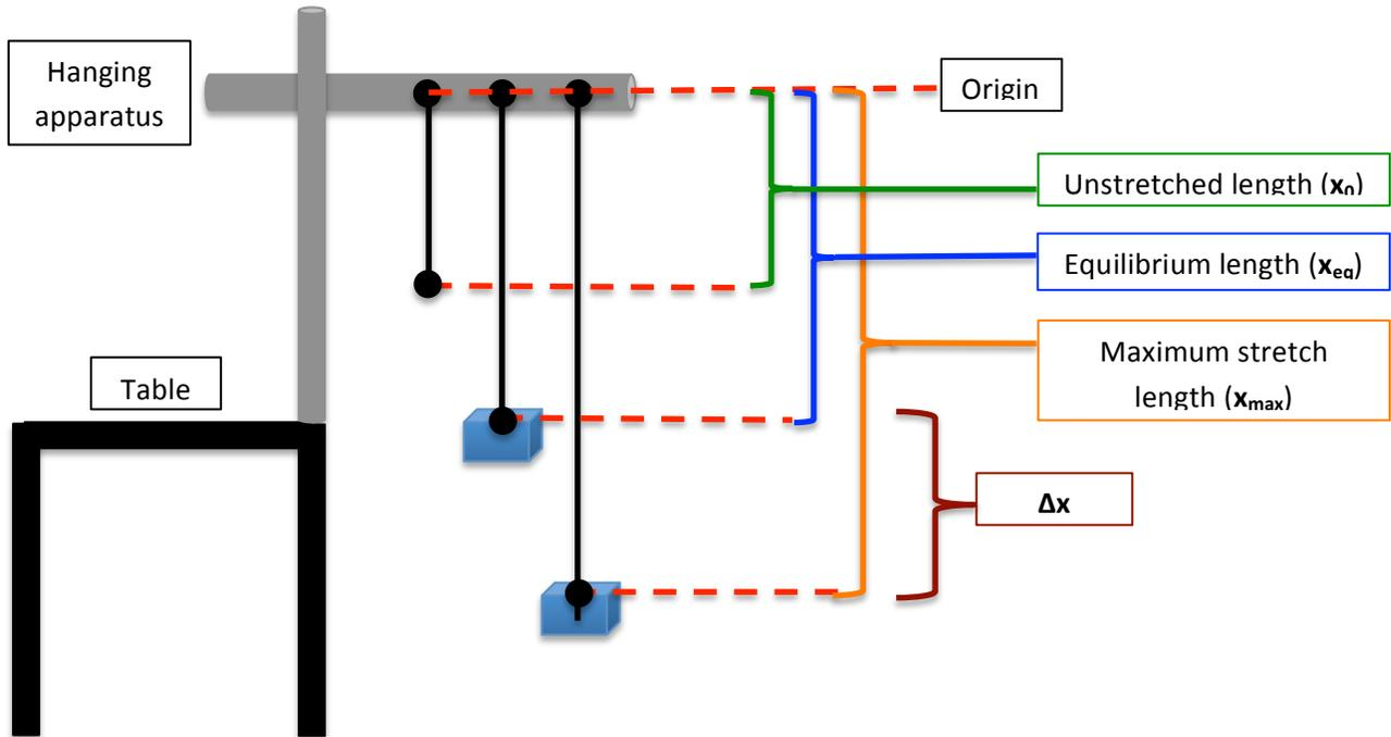
Figure 1: Diagram of the bungee cord experimental setup, where  $x_{max} - x_{eq} = \Delta x$  (eq. 2).
