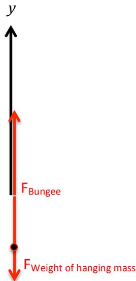
Figure 2: Free body diagram of the bungee system
