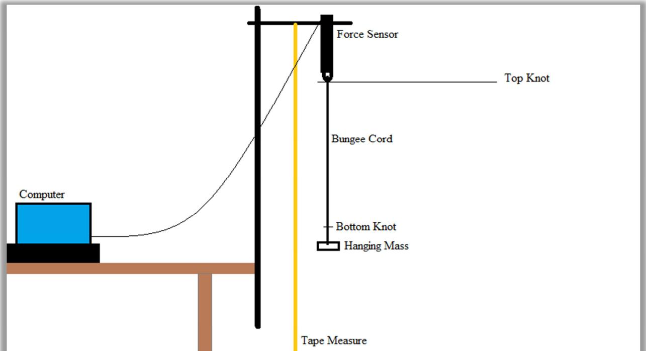
Using an arrangement of metal poles and vices, we suspended a force sensor and a tape measure from a horizontal pole approximately three meters off the ground. We attached lengths of bungee cords to a force sensor at one end and to a .150kg weight at the other. The original length of the bungee cord was determined by the distance between the top knot attaching it to the force sensor and the bottom knot attaching the weight to the bungee.
