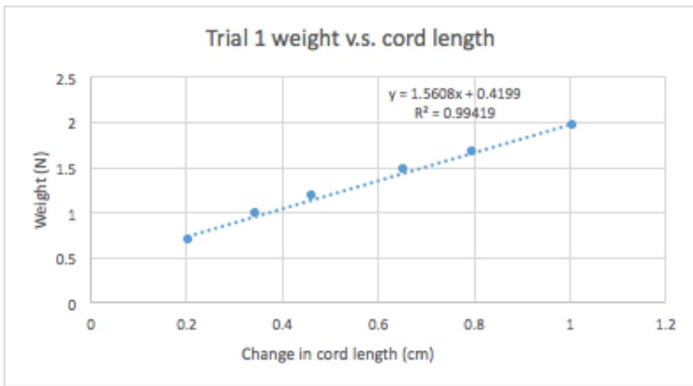
This graph is essentially a form of Hooke's law, where weight (force) is plotted against  $\Delta x$  and the slope is K. This models  $F_{\text{spring}} = K \cdot \Delta x$ . Notice the  $R^2$  value of close to .994 tells us the data is sound.
