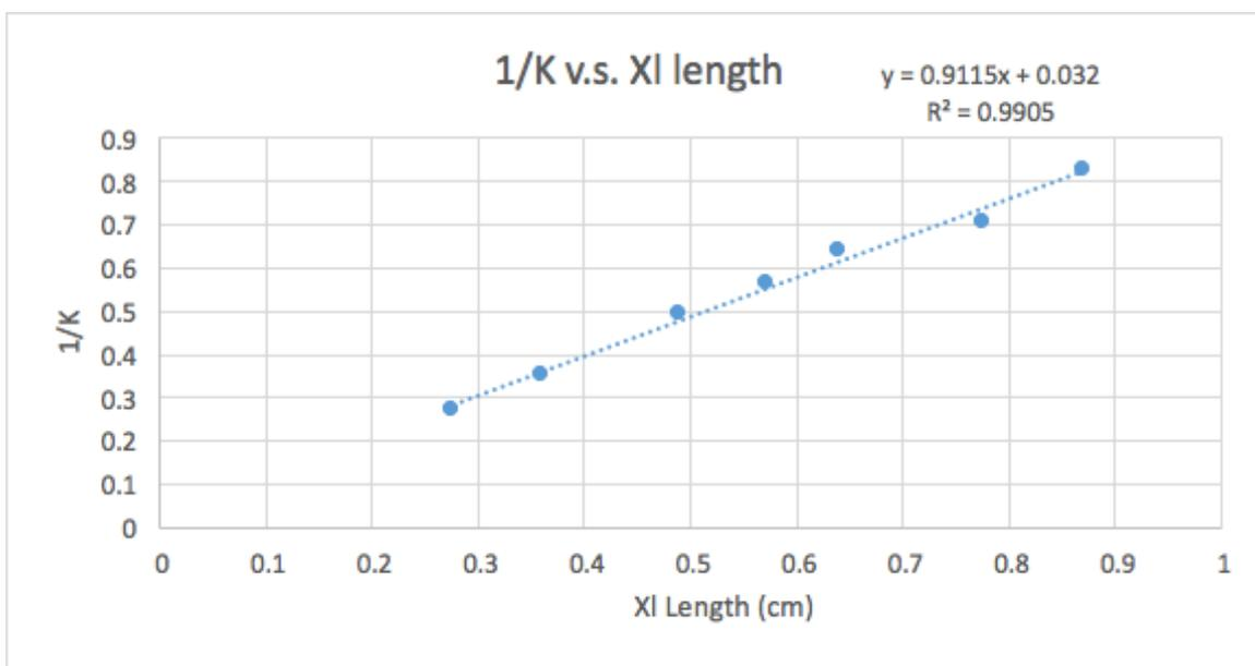
The Hooke's law relationship  $1/k$  v.s. length can be taken advantage of here in linearizing our data in Graph 2. Linearizing our data makes this far easier to perform regression analysis and find the error associated with slope and y-intercept.  $R^2$  value of .9905.
