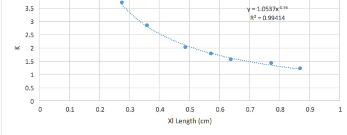
Here we have K plotted against a given cord length. As noted in the procedure section, we performed seven trials in order to find seven different K values at varying lengths. This allowed us to build this exact graph above where we can now see how K behaves when length increases or decreases. As length increases, k decreases and vice versa (although not linearly).  $R^2$  value very close to .994 and the exponent in the equation is -.96.
