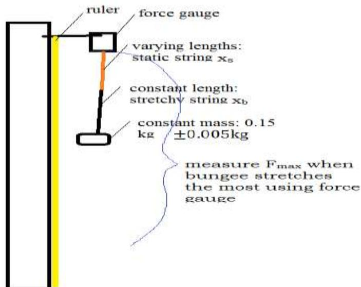
The static string is tied by a knot to a force gauge that will measure  $F_{\max}$ . The stretchy string is tied to the bottom of the static string, and the mass is tied to the stretchy string. A ruler will be beside our bungee system to help measure the length of the varying static string.
