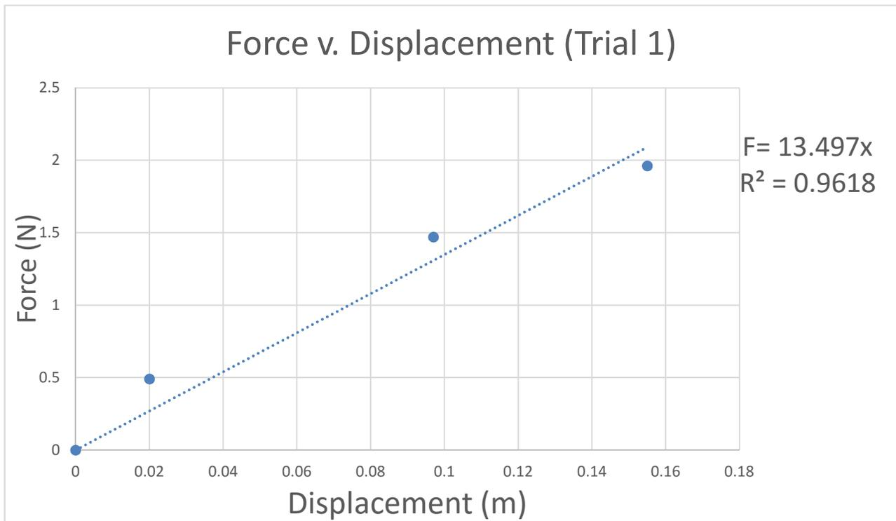
Graph 1. Force v. Displacement when the elastic band was .254 meters.
