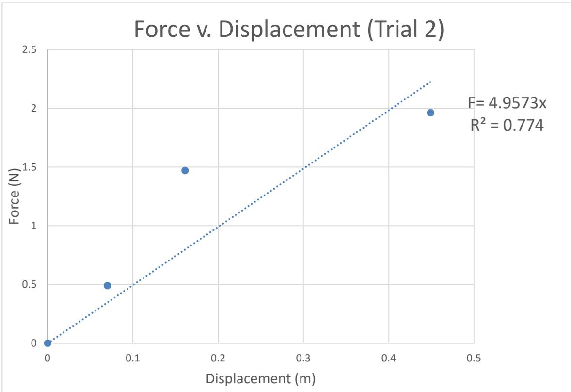
Graph 2. Force v. Displacement when the elastic band was .741m.
