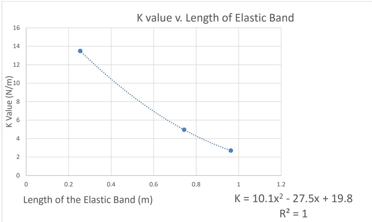
Graph 4. K value v. Length of the Elastic Band. Using the function of length of the elastic band, we thought this function would be a good model for lengths closer to 9 meters.
