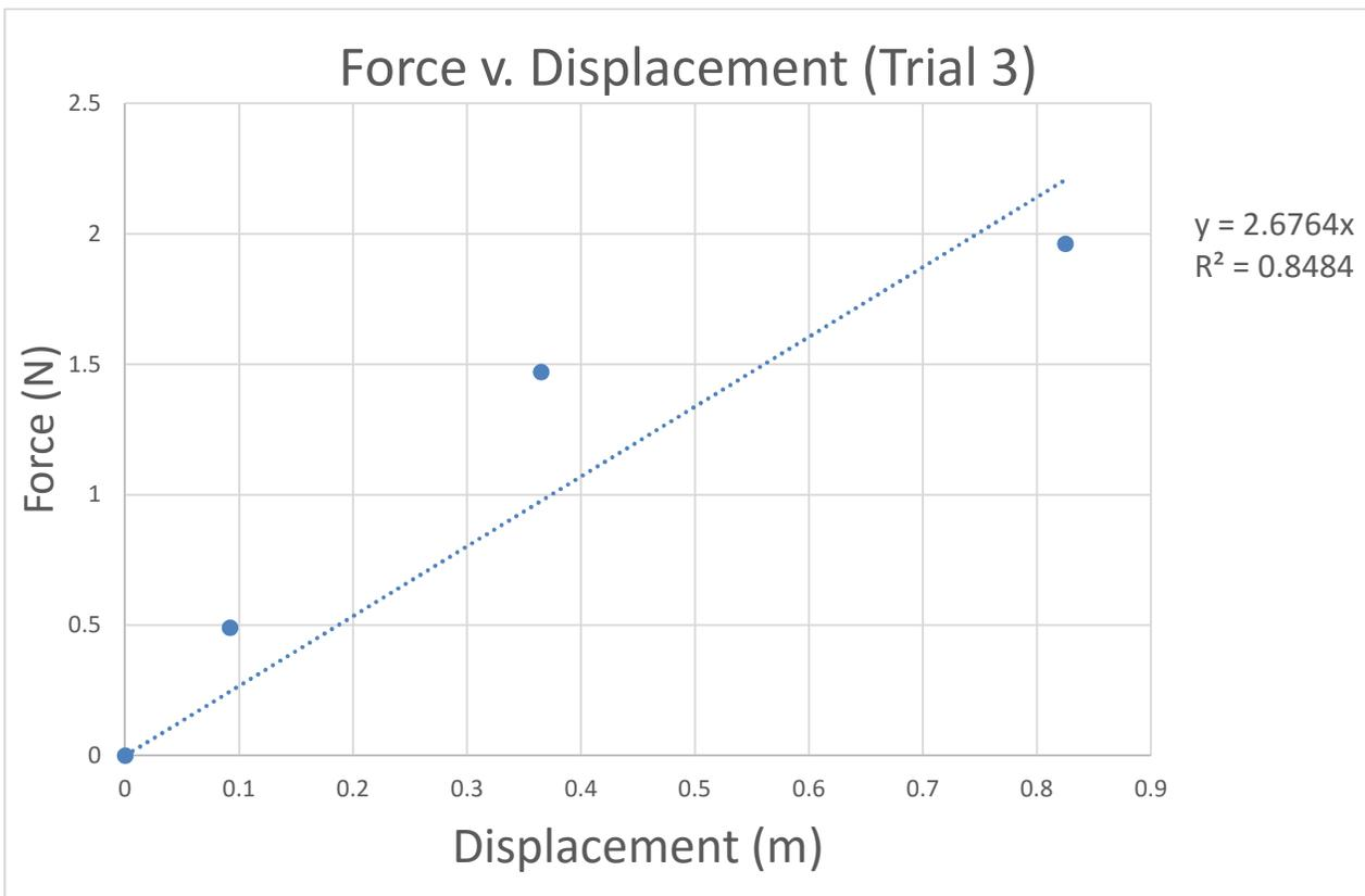
Graph 3. Force v. Displacement when the elastic band was .963 meters.
