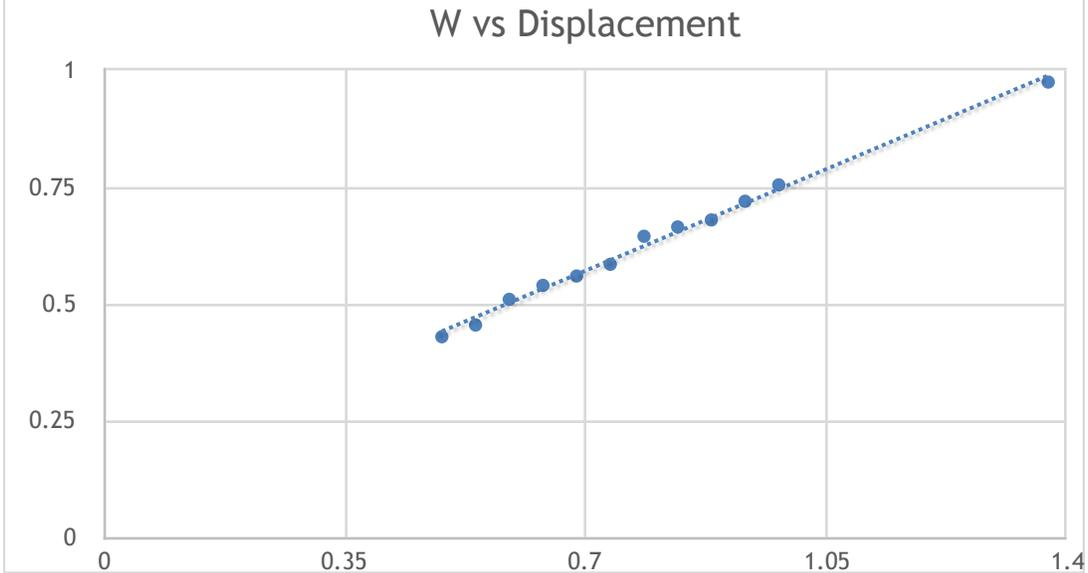
Figure #3: Relationship between Weight (mg) verse Displacement
