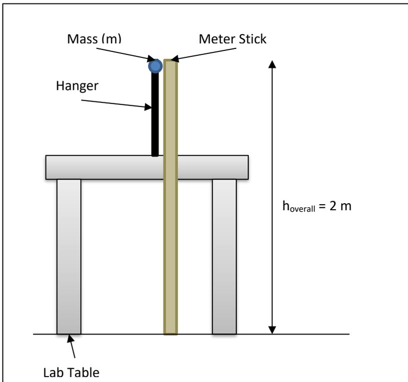
**Fig. 2: Experimental Setup during Drop.** The mass falls along the length of the meter stick and stretches the bungee cord.
