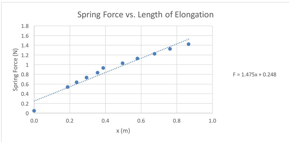
**Figure 3: Regression Analysis table.** The results of the regression analysis show the Spring Constant to be 1.475 ( $\pm 0.111$ ) N/m and the Intercept for the Spring Force equation to be 0.248 ( $\pm 0.056$ ) N. This gives us the equation of the Spring force to be  $F_{Spring} = 1.475x + 0.248$ , where x is the change in length of the bungee cord from the original measure.
