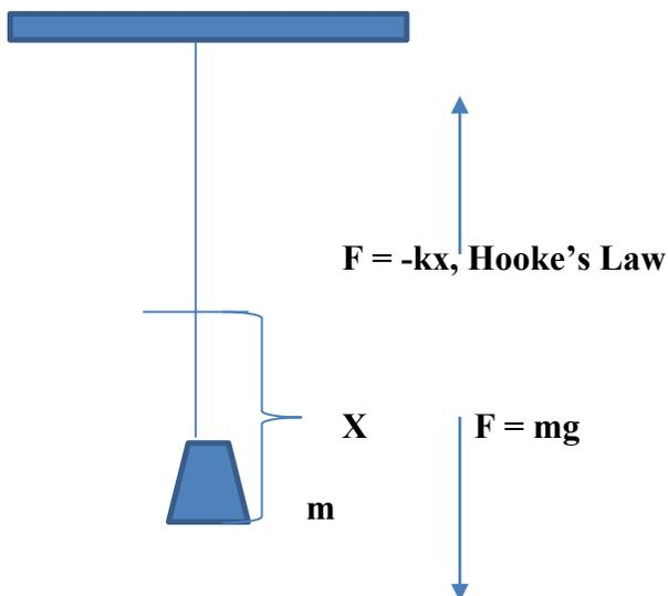
**Figure 1, Experimental Design** – The mass starts at rest from the top of the system and falls from there until  $x$  length past equilibrium length.
