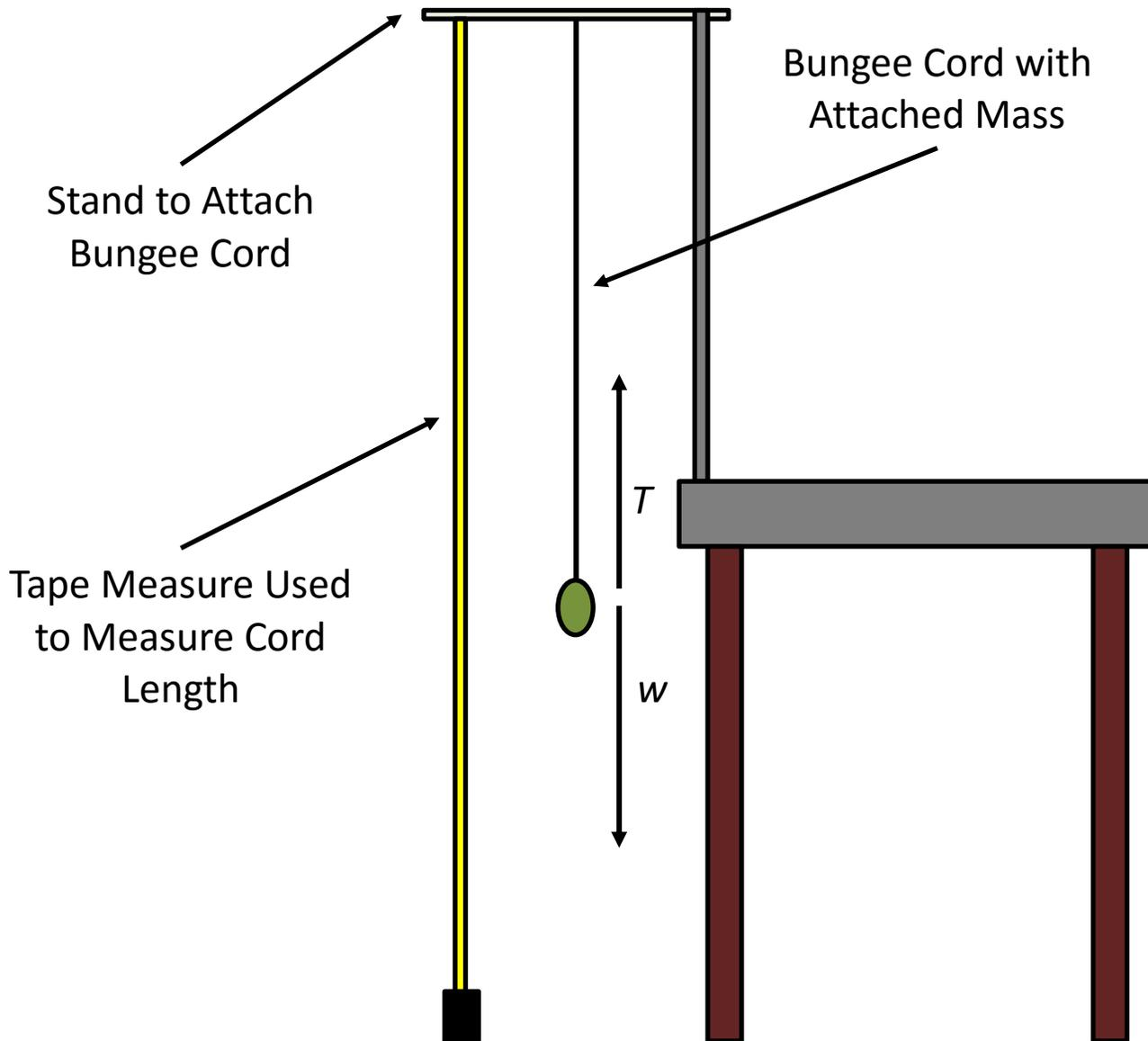
Attached to a table was a stand to which the bungee cord was tied. Attached to the same stand was a tape measure used to measure the length of cord after each drop. The mass was released from a point level with the stand.
