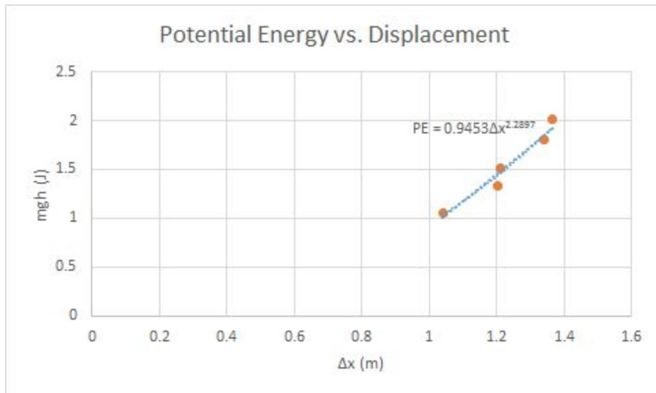
Figure 2: Relationship between potential energy and cord displacement for varying masses.
