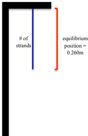
**Figure 1:** Prior to measurement, the number of strands, one, two, or four, were attached to a horizontal bar at a constant equilibrium position. The equilibrium set in this experiment was 0.260m.
