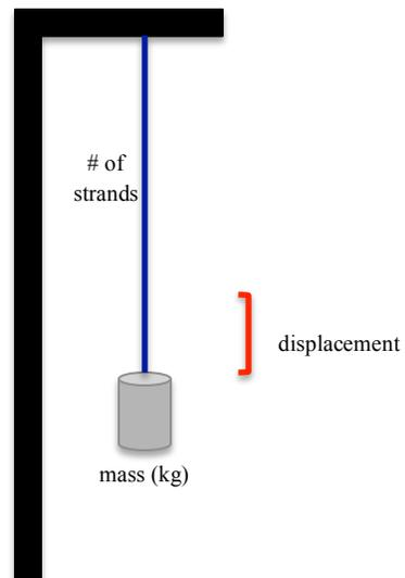
**Figure 2:** Once the mass was hung from the end of the strand(s), the displacement from the equilibrium position was measured and recorded. Five different masses were tested for each number of strands.
