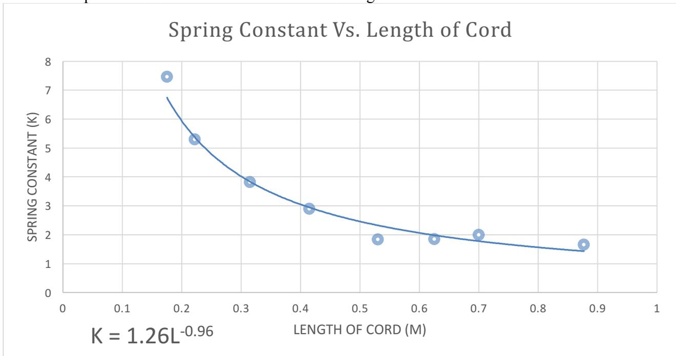
**Fig. 12: Spring Constant vs. Inverse Length of Cord.** The graph was linearized in order to fit the equation so that the spring force, K, is equal to the force times the inverse length.
