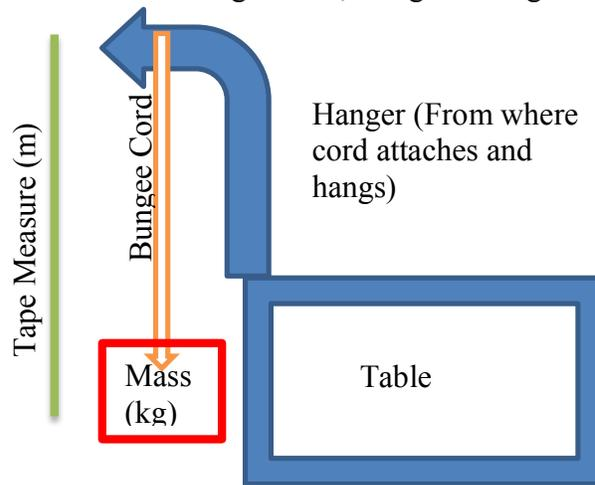
A hanging mass was attached to the bottom of the bungee cord of length  $l$ . The cord was taped to a hanger so that the mass would not hit the ground when the cord stretched. A tape measure was used to measure the length of the cord, both with the hanging masses, and without them.
