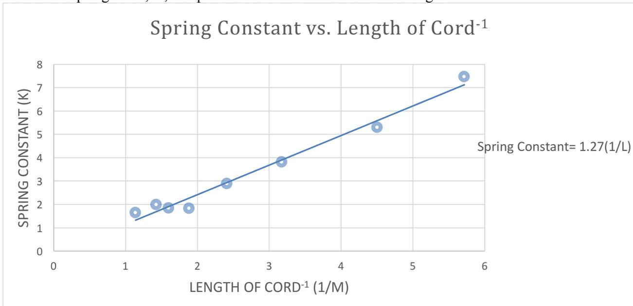
**Linearized equation:** Spring Constant (K) = 1.267(1/L) with a .074 (or 5.83%) uncertainty in the slope coefficient.
