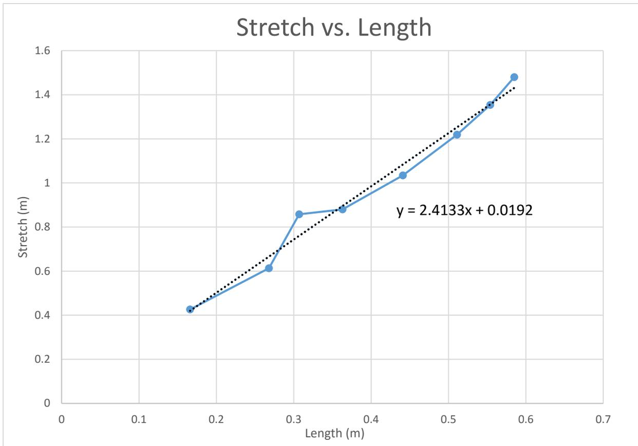
**Figure #3: Length vs. Stretch.** Graph depicting the semi linear correlation between the actual length and the net stretch it experiences when a mass is attached and dropped from the height of the connection point of the cord.
